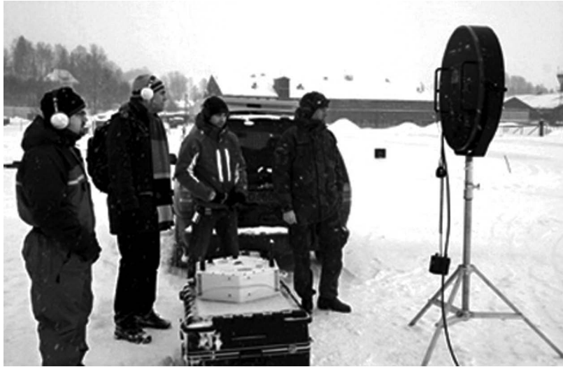
Figure 9 LRAD 1000 on tripod during a test by the Norwegian Defence Research Establishment (FFI) in April 2006. 164 The hexagonal object on the box in front is the smaller LRAD 500. (Photo reprinted by courtesy of FFI)
